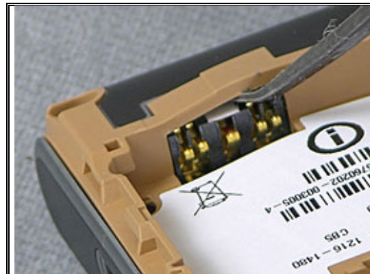
Location of the liquid intrusion indicator
